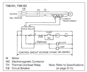
The TSB151 and TSB152 series SHOCK RELAY allows easy connection into new or existing applications. For single or three phase motors, simply wire the current transformer that we supply into one line of the motor and the SHOCK RELAY into the control circuit (stop-start circuit).
